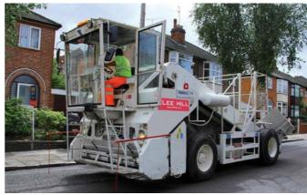
Clee Hill Plant's extensive fleet of pneumatic tyred rollers includes machines in a range from 4 to 28 tonnes. The larger machine's operating weight to the application. Due to their excellent kneading effect, pneumatic tyred rollers achieve an excellent sealing of the surface. Pneumatic tyred rollers are used on applications such as highway and airfield maintenance, the compaction of cementitious materials and surface dressing.
