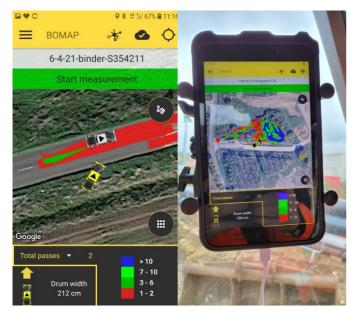
The operator can view compaction progress, pass counts with optional display and recording of the compacted soil stiffness on an easy-to-use colour display through a tablet.
