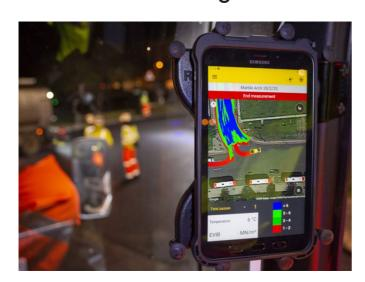
The system can also use GPS data, from one or more machines, to enable the location to be stored electronically together with the asphalt temperature and number of passes for future reference.
